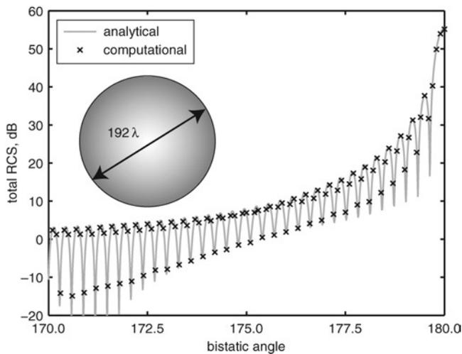
**Fig. 1** Bistatic RCS of sphere of radius  $96\lambda$
