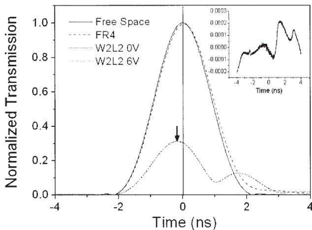
**Figure 3** Pulse waveforms in the time domain. The solid line is the reference (incident) pulse, and the short dashed and dotted lines denotes the pulse train through power-OFF and power-ON OLEDs measured by the receiver, respectively. The dashed line denotes the result of the pulse passing through FR4 sample. The insert shows the difference between the power-ON and power-OFF cases (6V-0V)
