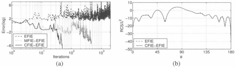
Fig. 3. (a) Comparison of convergence characteristics of the EFIE, the MFIE-EFIE, and the CFIE-EFIE formulations using BDP. (b) Normalized radar cross section ( $\text{RCS}/\lambda^2$  in dB) on the  $z$ - $x$  plane with respect to  $\theta$ .
