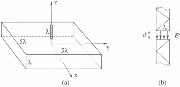
Fig. 1. (a) Composite geometry involving a dipole antenna (open surface) of length  $\lambda$  located over a perfectly conducting rectangular box (closed surface) with the dimensions of  $\lambda \times 5\lambda \times 5\lambda$ . (b) Delta-gap source located at the center of the antenna.
