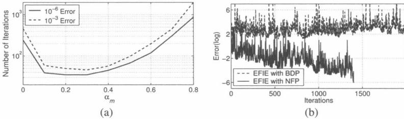
Fig. 2. (a) Iteration counts for the solution of the radiation problem in Fig. 1(a) with the CGS algorithm with respect to the value of  $\alpha_m$ . (b) Convergence characteristics of the EFIE formulation using the BDP and NFP to accelerate the iterative solution.
