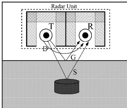
Figure 1: The typical GPR problem and the GPR configuration with a transmitter and a receiver.
