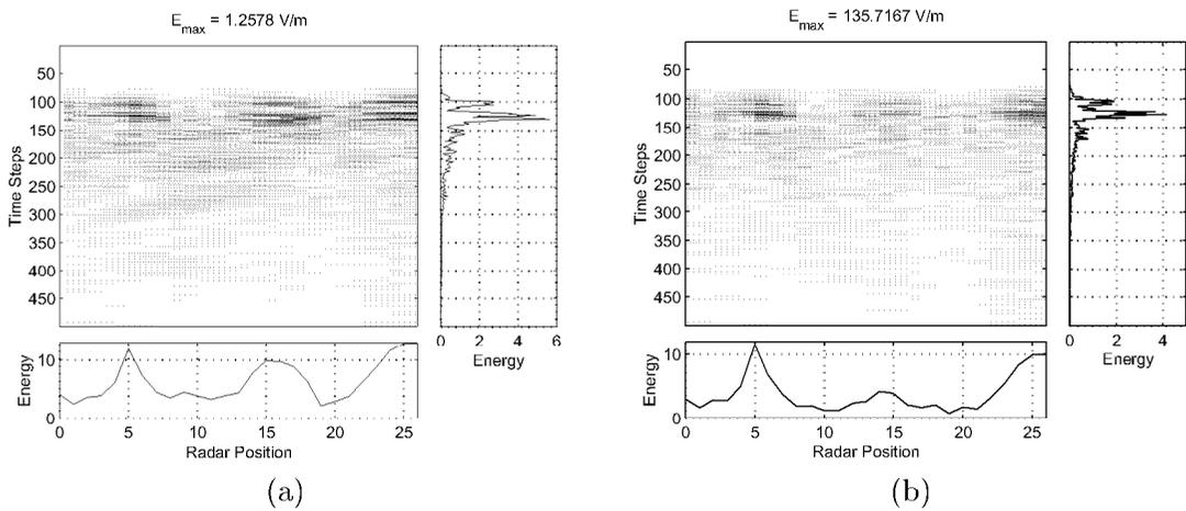
Figure 6: Simulation results of a conducting disk, buried under a ground with conductivity 0.6 S/m, obtained at (a) 200 MHz and (b) 1000 MHz center frequency.
