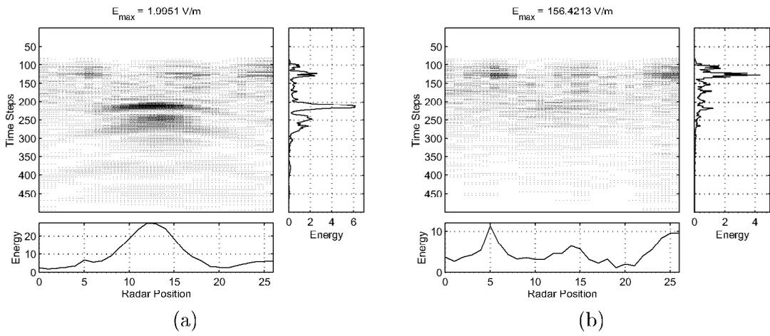
Figure 5: Simulation results of a conducting disk, buried under a ground with conductivity 0.2 S/m, obtained at (a) 200 MHz and (b) 1000 MHz center frequency.
