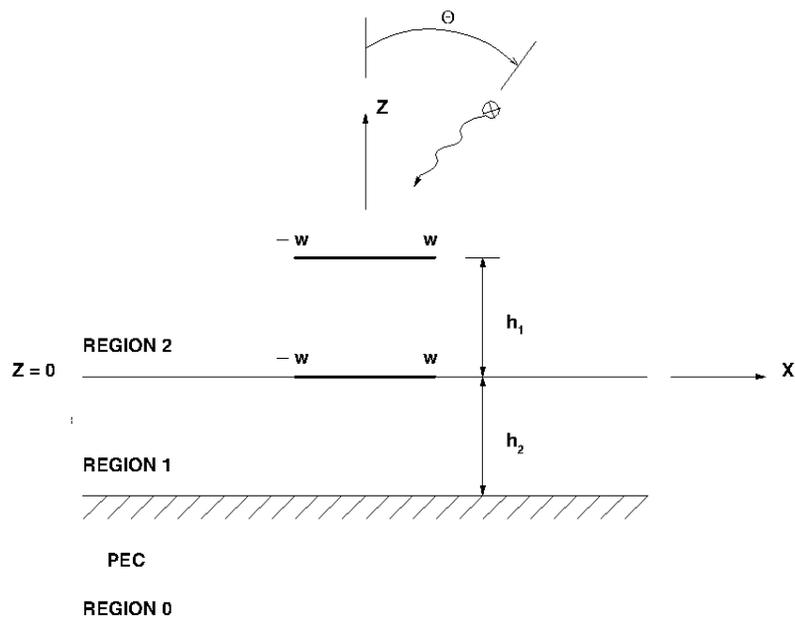
Figure 1: A two-strip, three layer geometry.
