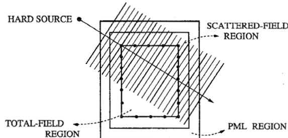
Figure 1: Excitation of a three-dimensional FDTD grid using a one-dimensional incident-field array.
