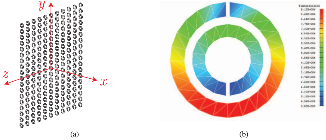
Figure 1. (a) Single-layer SRR array obtained by the arrangement of 11 \times 18 SRRs. (b) Induced surface current on a single SRR at 90 GHz.
